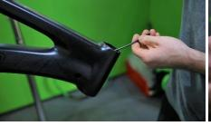
5)Feed the cable until it appears out of the head tube top cup.
