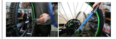
Using the 8mm allen key, insert it through the frame and hub. Apply a bit of pressure and wiggle if necessary, until the axle locates in the hanger Using an 8mm allen key, turn the axle clockwise until it bites. Use a torque wrench to set the axle to the correct setting - 30-35Nm
