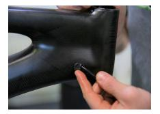
Push the grommet into the hole, allowing the groove to sit flush into the frame.
