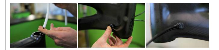
7)Slide the foam tube onto the cable and push until it fully disappears inside the frame. 8)Push the cable back into the frame and then feed it through the drive side hole. 9)Slide the single hole, larger size rubber grommet onto the cable and wiggle it into place. The groove on the grommet should sit inside the frame.
