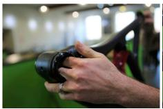
4)Using your fingers, guide the cable round the BB and feed it up the down tube.
