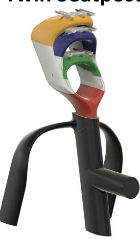
In combination with a common base (red) and three seatpost head sizes (yellow, blue green), configurable upright elements (grey) allow custom saddle position.
